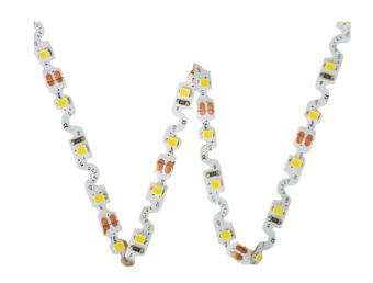
The flexible LED strip is convenient when assembling letters and other products of complex shape. It can be bent at an angle of up to 90 degrees. A narrow lining of 6 mm allows you to install aluminum profiles. Available in all colors in 5m spools.
